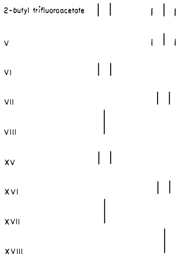
Figure 1. Schematic representation of the NMR spectra of the methyl regions of the solvolysis products.
